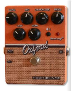
Sabbath-like grind, or a modern, high-gain lead tone. Its three-band equalization circuit is supremely useful, and Tech 21's switchable speaker simulation (which emulates a 4x12 loaded with Celestion Greenbacks) makes the Oxford perfect for recording direct, or running straight into the PA when playing live. For realistic, direct-to-the-board Orange tones, one cannot do better than the Oxford.
