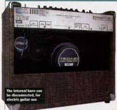
reveals the slightly offcentre mounted 12-inch driver and top-right mounted horn obviously Tech 21 gets these made elsewhere, but keeps the manufacturer under its hat.
