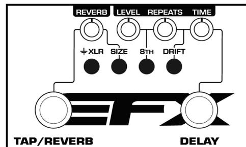
**Repeats Tip:** When using the Delay in front of an amp, the amp will compress the signal and the repeats will become more pronounced. Therefore, you will most likely need to have the setting lower than you would when running through an effects loop. For instance, you may find a Repeats setting at 10 o'clock through an effects loop will yield 3 repeats. However, through the front of an amp, you may find a setting of 8 o'clock will give you the same results.
