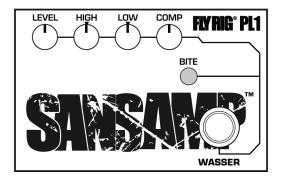
**COMP:** A single, continuously variable control to dial in just the right amount of compression you need. A little goes a long way, from soft and barely noticeable to super squashy, infinite sustain. Utilizes old school, all-analog, FET-based technology from the '50s and '60s, which is inherently warmer, more transparent and more musical than other methods of compression.
