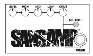
**DRIVE:** Adjusts the overall amount of gain and overdrive, similar to when the output section of a tube amp is being pushed.
