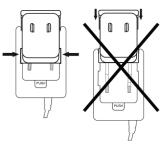
Press the PUSH switch to release the prong assembly. Slide the assembly up (about halfway) to align the side tabs of the prong assembly with the slots of the power supply housing. Then pull up
